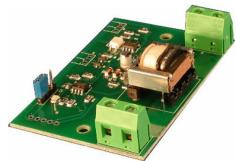
The "Block Watcher <sup>™</sup> has many uses and applications. It can not only be used as the basis of signaling systems, but can also be used to indicate occupied blocks or triggers
